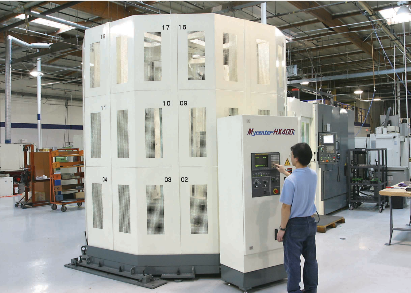
View of Roberts Tool Company's new Kitamura HX400i 4-axis horizontal machining center. 21 palletized work settings (400mm pallets) can be brought into the machine automatically and stored for future call up. Programmable probing for tool, part, and fixture measurement assures precision every time work flows into the cell for machining. Tool storage capacity of 150 tools allows back up and redundant tools. Roberts can put as many as 60 jobs on the system at a time.
