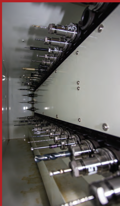
Left - Tooling carousels of 60 and 100 tools were a selling point of the Kitamuras. Right - The 5 axis machines can take a raw chunk of metal and do in one op what might have taken 2 or 3 ops on a 3 axis machine.
