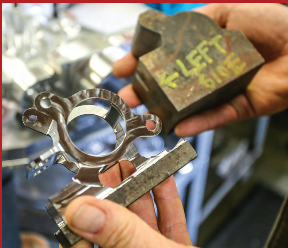
Left - Tooling carousels of 60 and 100 tools were a selling point of the Kitamuras. Right - The 5 axis machines can take a raw chunk of metal and do in one op what might have taken 2 or 3 ops on a 3 axis machine.
