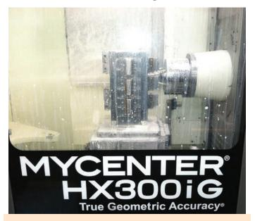
JLP employs a lot of dovetail workholding. "We manufacture our own dovetail fixtures from 17-4 PH stainless steel and then heat treat them to H900 for longevity," said Libby. "The Mycenter-HX300iG at JLP is utilizing the Renishaw NC4 laser non-contact tool detection and the OMP 400 spindle probe. After implementing these on previous machines, JLP will never buy another machine without them. The ROI is almost immediate in a job shop."
