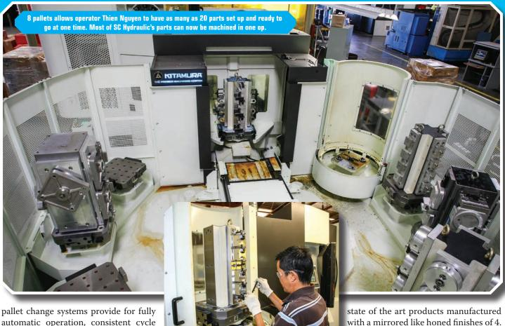
automatic operation, consistent cycle time and ±0.001" positioning accuracy. Speed and accuracy are key elements to SC's precision made pumps. With 8 pallets and 200 tools they can set up 15-20
