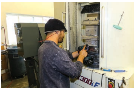
With a full time team of six running 5 machines it is packed in tight at Odenthal Manufacturing. A pair of Kitamura HX300 Mycenters lead the way with their full 4th axis capabilities. They also have a Fanuc Robodrill T14A, Boston Digital BD 22, and OKK PCV-40 to keep the two shifts always cutting.
