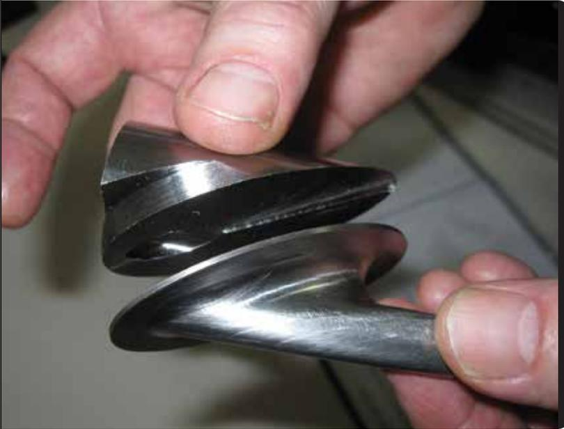
To permit enough access to the part so that most or all of its features can be machined in one setup, parts are often clamped via back-bolting. This part machined out of bar stock is cut away from the bolted portion of the stock as the final step in the cycle.
