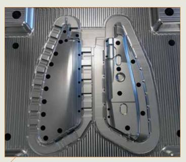
The Kitamura 4XiD's Arumatik-JR controller and 675 look-ahead allowed this core side of an aluminum prototype for an airbag cover that goes under a car's steering wheel to be machined in just three days, including unattended machining. This same job would have taken several weeks on the company's smaller CNC machine.
