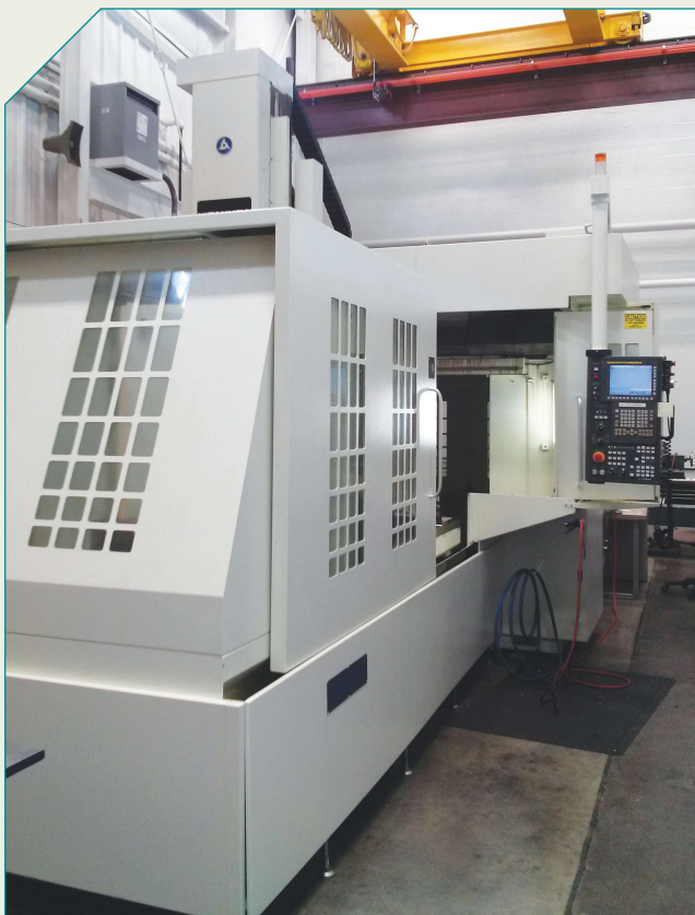
With a maximum table load of 13,200 pounds, the Bridgecenter 10 provides additional capacity and power for heavy roughing of larger molds.
