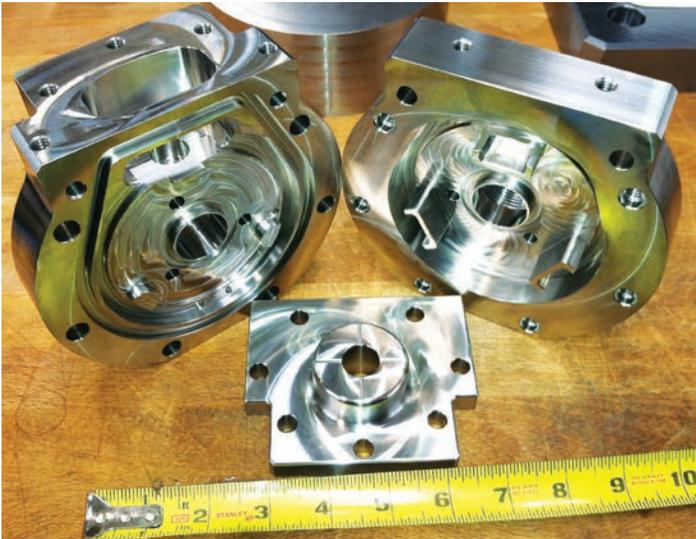
The components for which the Mycenter-HX300iG was purchased to machine are cut from 6.5 inch diameter 316 ss.
