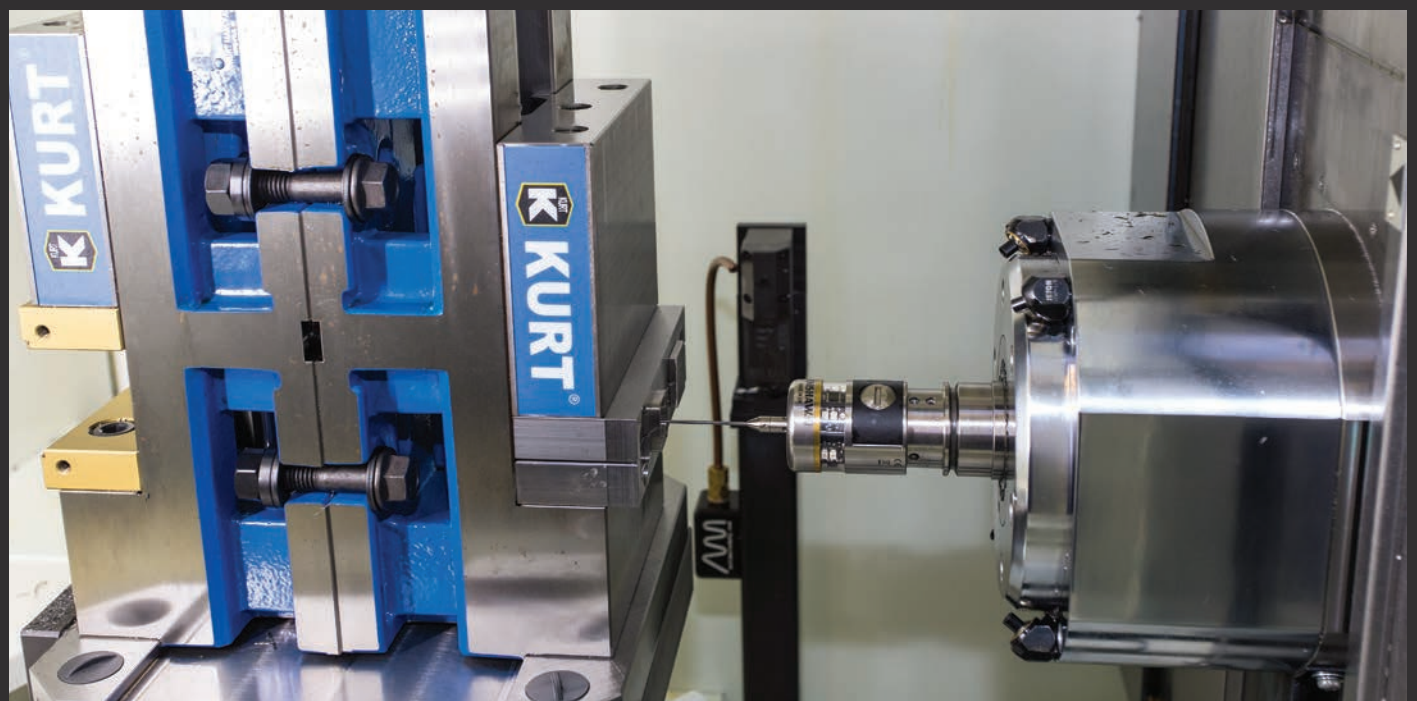
Josh added the Renishaw OMP400 probing system to his new Kitamura. He finds it invaluable on the watch parts because of size variance. Thickness on these tiny parts can vary by .004" on a .020" thick part. So with the Z axis probe he is getting no variance. With a .004" cosmetic chamfer or .007" pocketing there is no room for error. His only current non watch job is based off of casting and he has to probe every one before machining. He was doing it by hand before and it would take 5 minutes each. Now it is literally 30 seconds. Also on the machine is a BLUM laser system for tool measurement.
