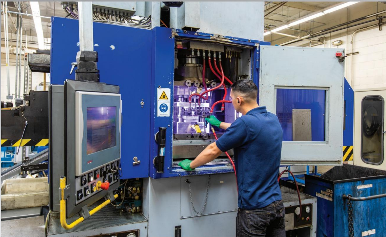
Fine blanking uses counter pressure to extrude the material as opposed to just shearing it. Fine blanked parts require less secondary machining.
