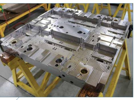
Dynamic Tool uses its two Kitamura Bridgecenter 6G#40 machining centers to fabricate these highly customized mold bases. The B-plate shown above is part of a production mold that produces filtering components for a medical device. Tooling techniques like cam actions, slides, lifters, auto-unscrew, in-mold closing or core toggle require sophisticated A- and B-plates manufactured accurately, efficiently and repeatedly. Source (All Images) | Dynamic Tool Corp.
