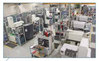
The Dynamic Tool team can repeatedly hold 5-micron/0.00020-inch tolerances on both hard-cutting and sinker EDMs. Not only is requisite equipment fitted with integrated CMM on the rail systems, but every component is 100% inspected before moving to the next operation. Shown above are Dynamic's sinker and wire EDM bays.
