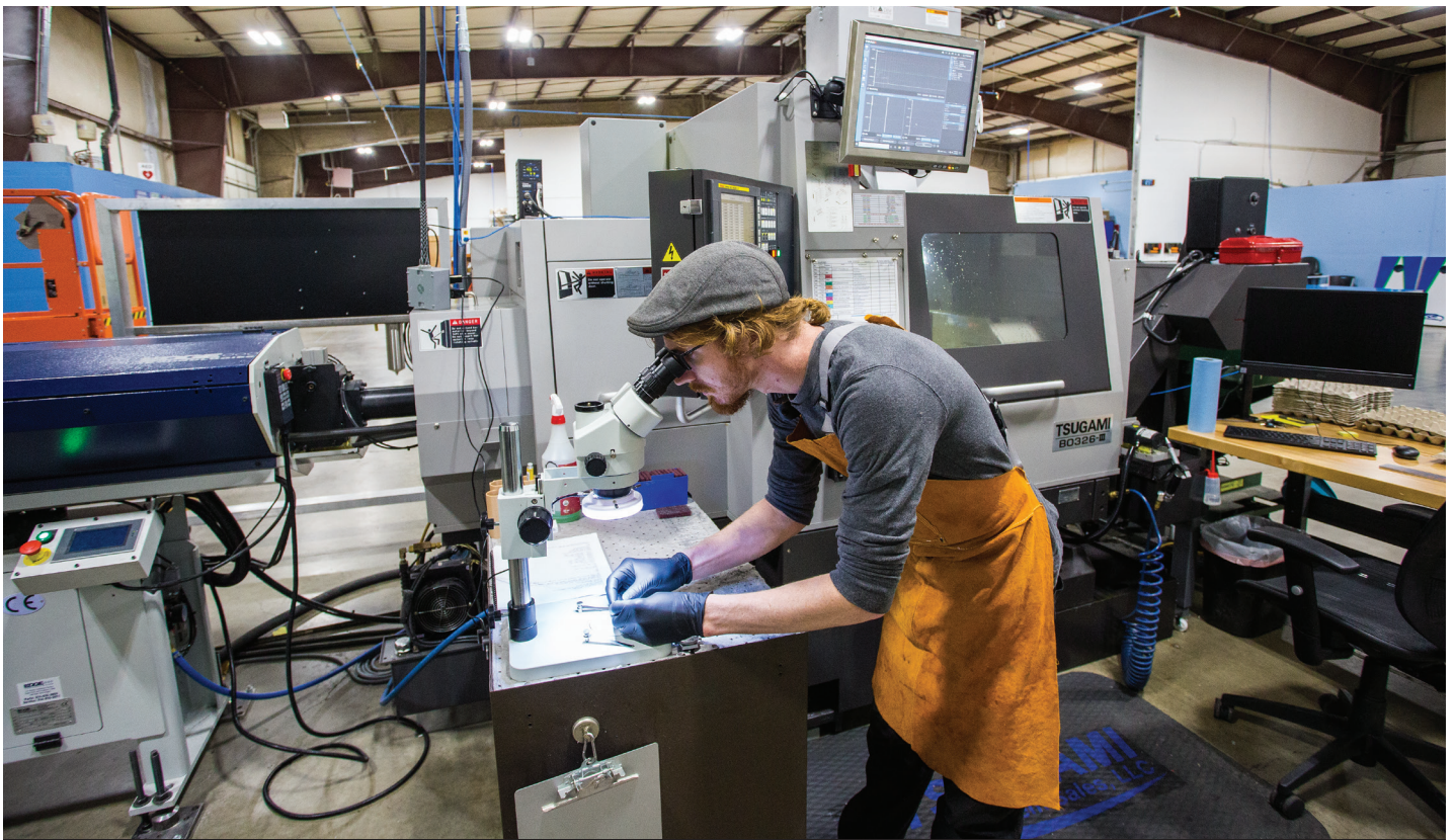
3V's Swiss turning department consists of a trio of Tsugamis all equipped with Caron Engineering's Tool Monitor Adaptive Control (TMAC) system
